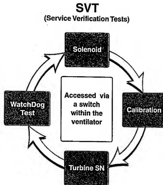
**Note:** During the SVT, Tidal Volume controls turbine RPM, Peak Flow controls turbine flow, PEEP/CPAP controls circuit pressure, and %O<sub>2</sub> controls the blender.
