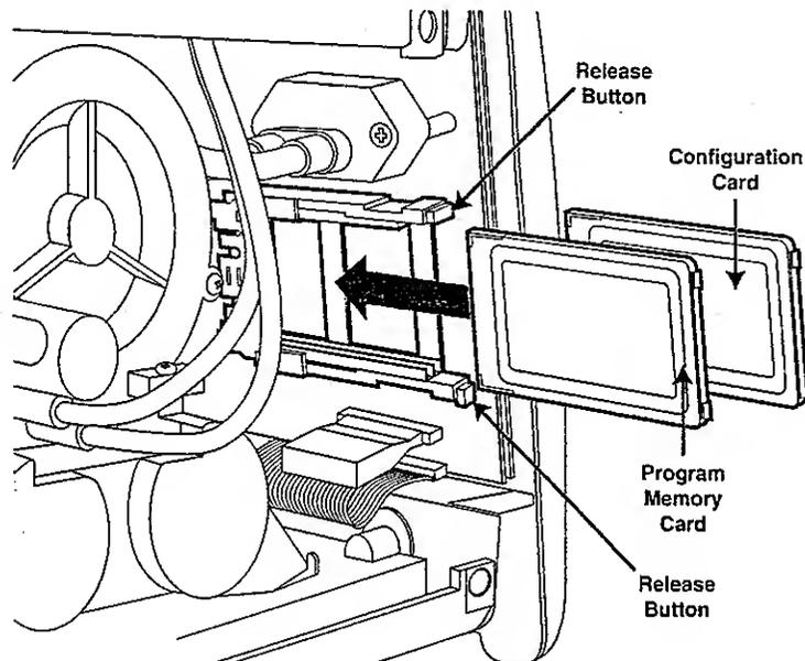
**Figure 5-3. Program Memory Card and Configuration Memory Card**
