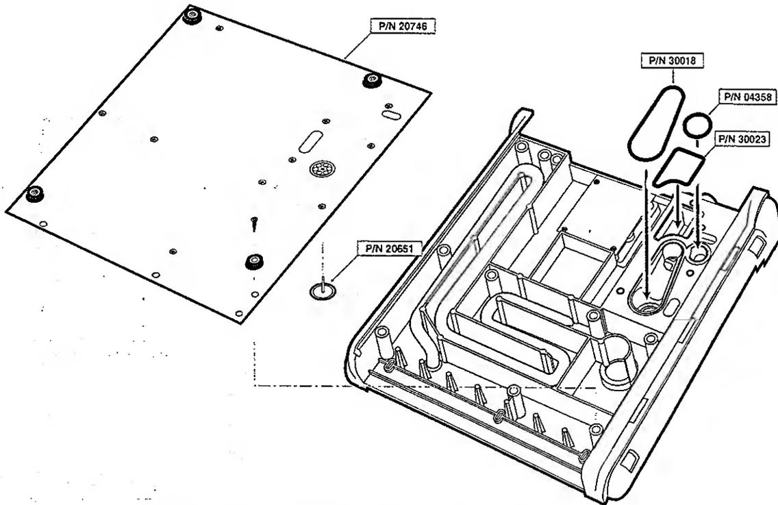
Figure 5-19. Base Plate O-Rings and Anti-Suffocation Valve
