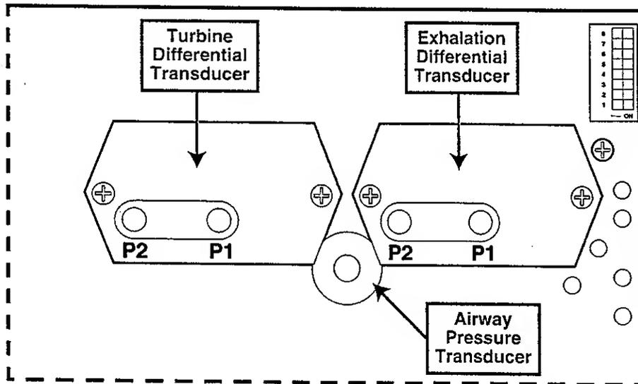
Figure 3-5. Airway Pressure Transducer
