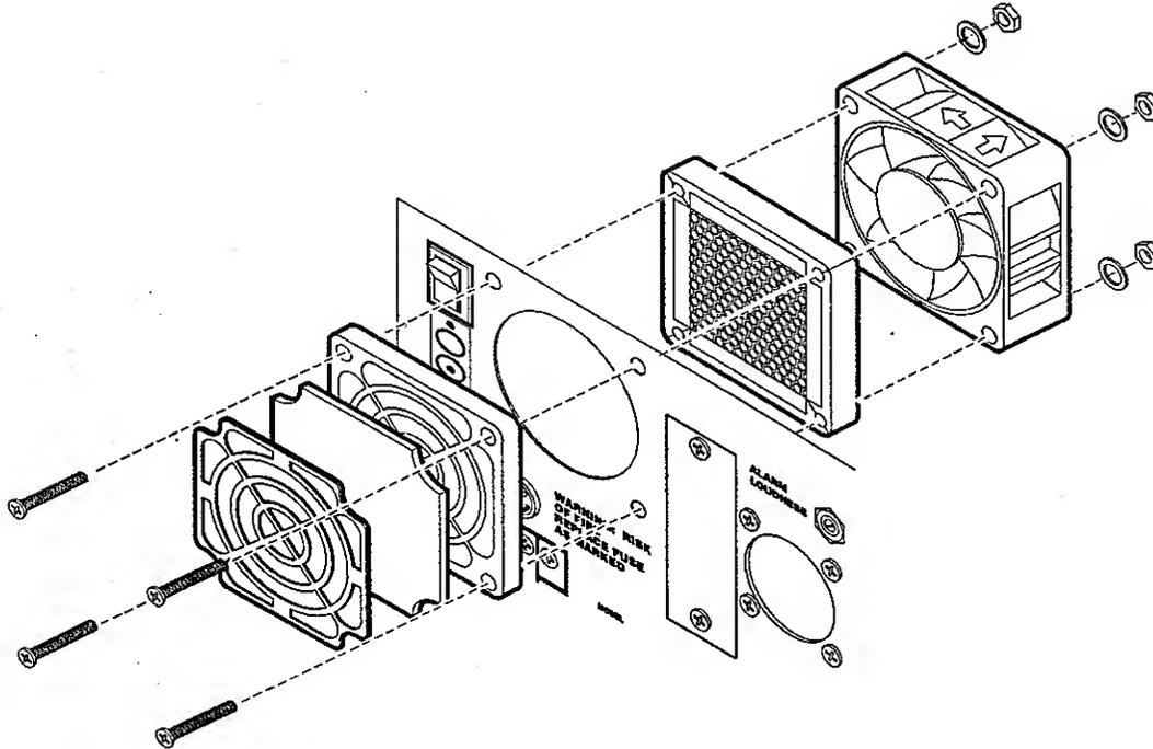
Figure 5-16. Fan Assembly
