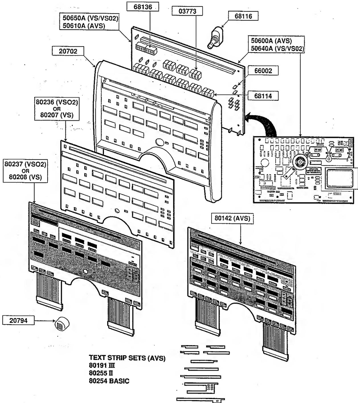
**Figure 5-9. Front Panel Disassembly**
