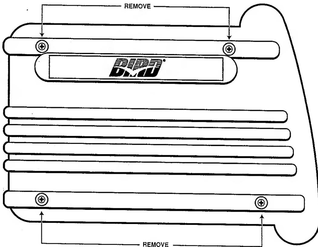
Figure 5-1. Ventilator Left and Right Side Cover Removal
