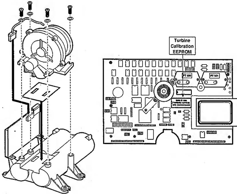
**Figure 5-14. Turbine Assembly**
