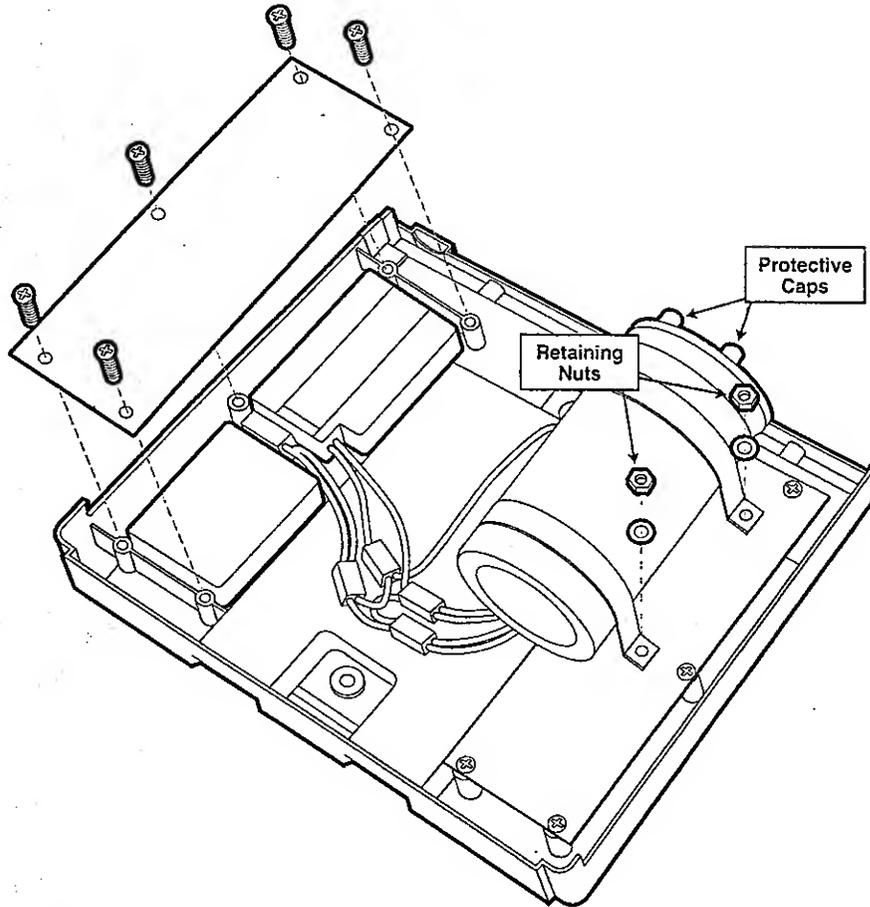
**Figure 5-6. Internal Batteries / Energy Storage Capacitor**
