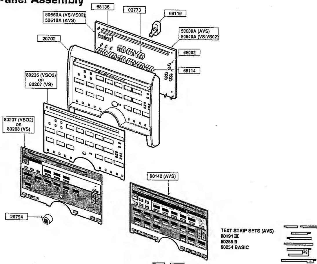
Figure 7-2. Front Panel Assembly
