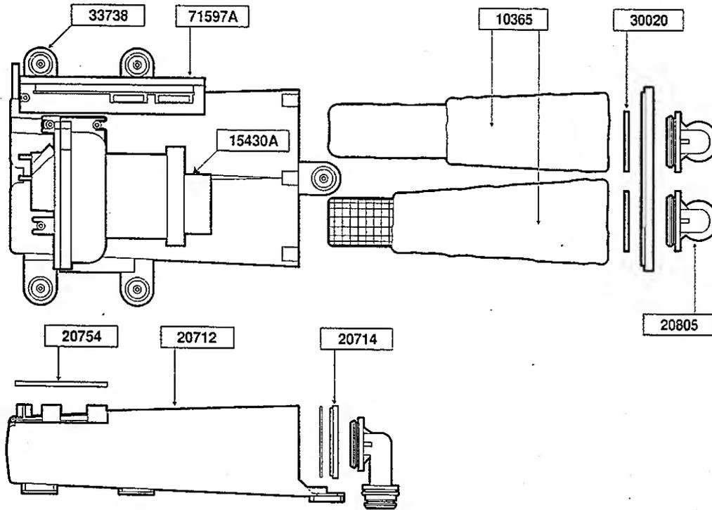
**Figure 7-1. Turbine/Muffler Assembly**
